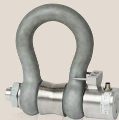
The F5302 is a load-measuring shackle for static and dynamic tensile force measurement. The force transducer is a high-strength stainless steel load pin with welded-on thin-film sensor elements. The dimensions and handling of the F5302 shackle correspond to those of standard shackles. Thus a universal application, even in existing systems, is guaranteed.
