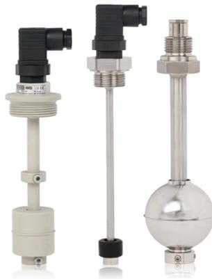
The RLS is a contact-free magnetic float switch for vertical mounting in medium to large vessels. It can be produced as normally closed, normally open or change-over contact with up to four switch points at individual heights. For the float, there are various geometries and materials available.
