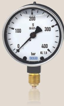
The model 213.40 Bourdon tube pressure gauge is fitted with a forged brass case. It is, therefore, extremely robust against mechanical loads. With its liquid filling it is suitable for use on measuring points with high dynamic pressure loads and vibrations.
