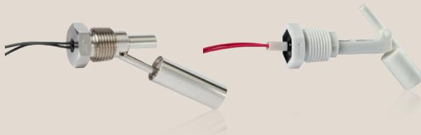
The HLS-M is a maintenance-free magnetic float switch with compact dimensions for lateral mounting in small to medium-sized vessels. It can be used as a normally closed or a normally open contact. The HLS-M can be made of stainless steel or plastic and is suitable for vessel mounting from the inside or outside.
