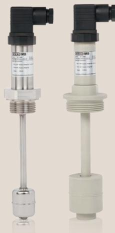
The RLT is a wear-free magnetic float transducer based on a measuring resistance chain for vertical installation in medium to large vessels. For the RLT there are various measuring lengths and measuring resolutions available, its float can be produced in different geometries and materials.
