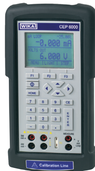
Hand-held multi-function calibrator model CEP6000
